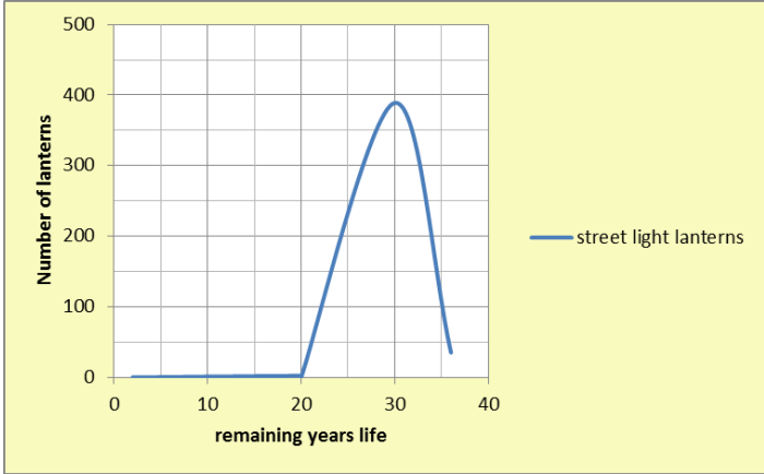
Chart 1: Expected remaining life of existing street light lanterns
