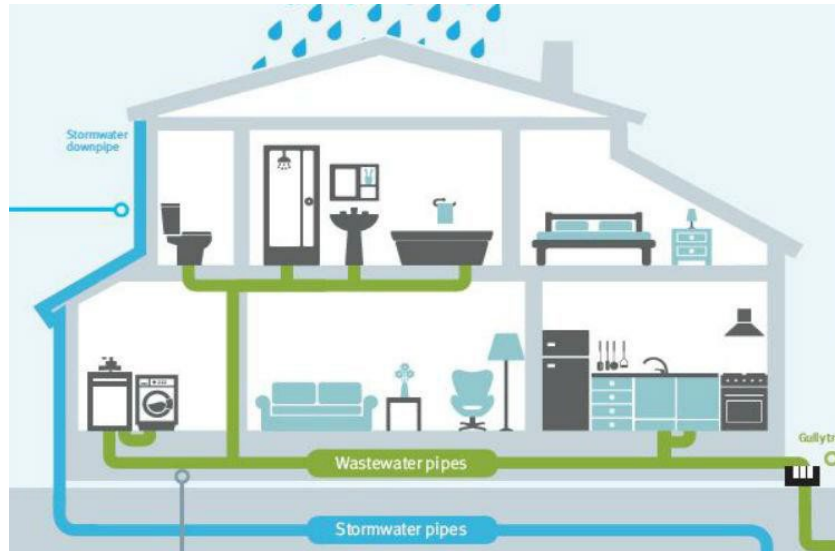
Figure 2.1: Wastewater and Stormwater Examples
