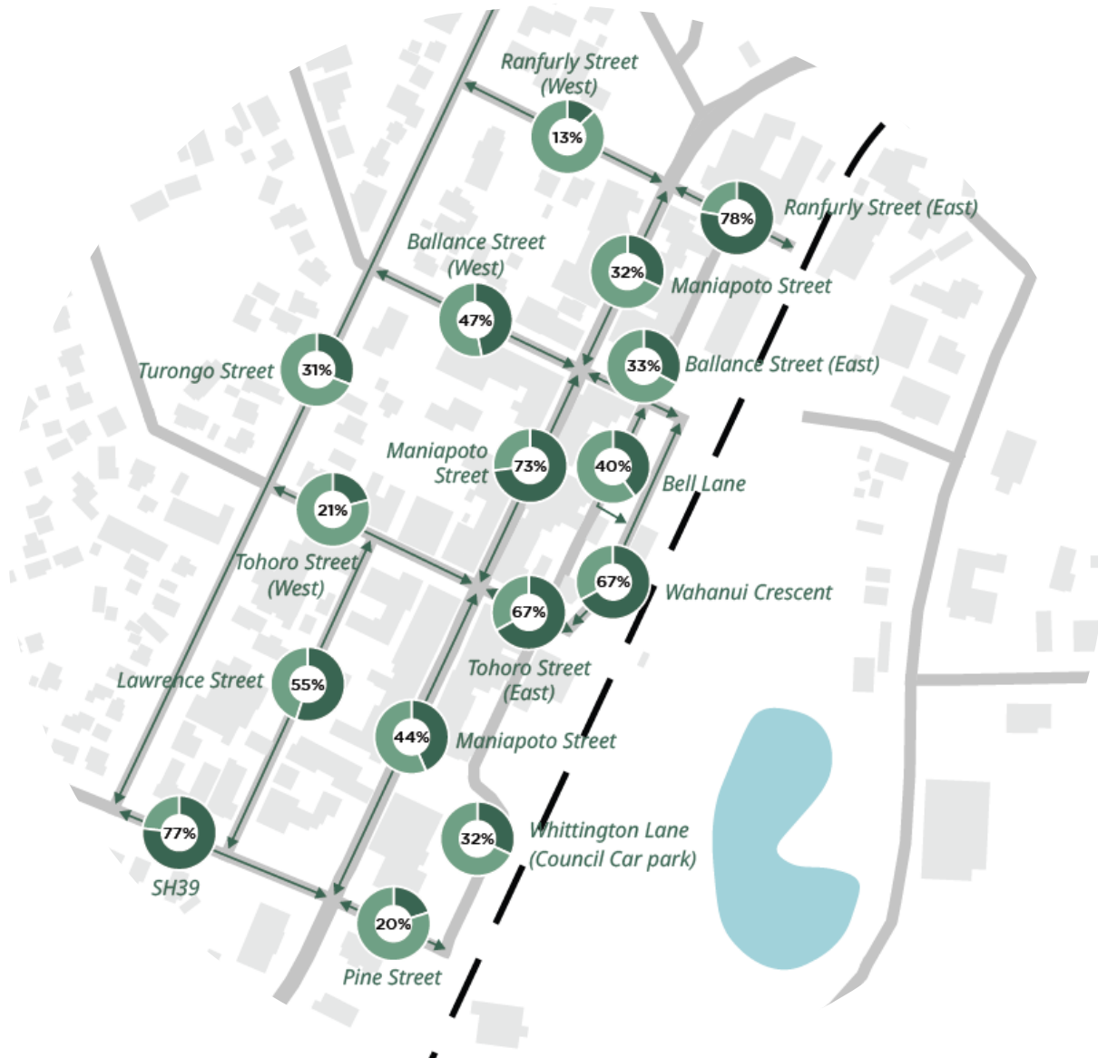
Figure 4 Average parking occupancy of the streets of Ōtorohanga town centre (Ōtorohanga Town Concept Plan 2022)
